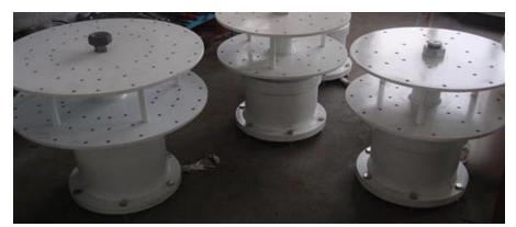
**Blades connector:** They are made of the mild steel plate and surface treatment is painting against decaying. It will connect the blades and the generator.
