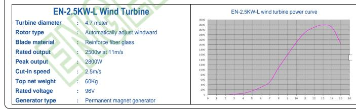
\* Wind turbine performance is subject to many factors. All output data contained in this document is indicative and actual turbine outputs will depend on the prevailing site and installation conditions.
